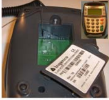
(a) A rigid wire is inserted through a hole in the Ingenico's concealed compartment wall to intercept the smartcard's data. The front of the PED is shown on the top right.
