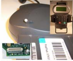
(b) A needle is inserted through the rear of the Dines PED for data interception, attaching to a ribbon cable connector shown on the bottom left; a mounted PED is in the top right.
